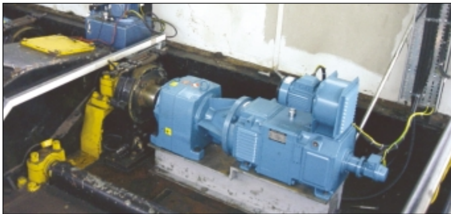
Thurlby Electric DC Motors with In-Line Gearbox
